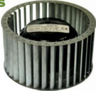
External rotor motor, PSC capacitor type. Single phase. Single speed. Metal tablock impeller. 2 pole (2550RPM). Diameter: 133mm, Class B. IP54 enclosure, -30'c to +60'c.
