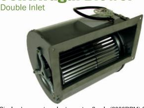
Single phase, external rotor motor. 2 pole (2300RPM) & 4 pole (1300RPM). 1 to 4 speeds. Class B & F. Wheel diameters: 120, 133 & 146mm. Lengths: 126, 180 & 190mm. Range of mounting flanges.
