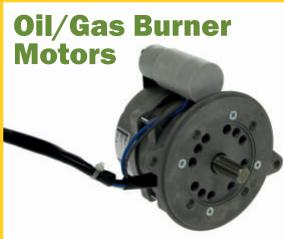
PSC capacitor motors, 2 pole (2800RPM), 50W to 250W. Class B insulation, mechanical duty. Pump drive coupling option, (32mm/54mm). 2 or 4 lug flanges. OEM specials & equivalents.
