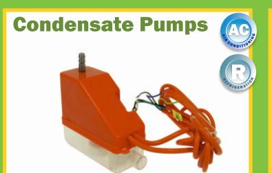
Single phase. Class II appliance. Class F insulation. Standard & EC models. 12m discharge head. 2m lift. Flow rate 12L/hr to 120L/hr. Intermittent duty. Maximum water temperature 50'c.
