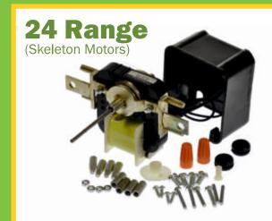
Open frame skeleton type shaded pole motors. 220/240V, 2 pole (2500RPM), class F insulation, fan hub or plain shaft, front or rear fixings, pedestal brackets, etc.
