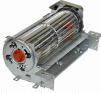
Shaded pole motors. Single speed. 2 pole (2500RPM), Class B & F. Impeller diameters: 30, 45 & 60mm. Lengths: 60, 90, 120, 180, 240, 270, 300, 360, 420, 480, 550 & 610mm. 0'c to +60'c.
