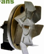
Shaded pole motors. 36W to 56W. 2 pole (2100RPM). Class H. High temperature bearings. Heat sink cooling fan on shaft. 150 & 160mm diameter paddle blade. Mounting plate or arms.
