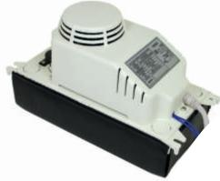
Single phase. Class II appliance. Class F insulation. Maximum discharge head 3m to 6m. Flow rate 108L/hr to 180L/hr. 745cc tank capacity. Intermittent duty. Low maintenance. Water max 50'c.
