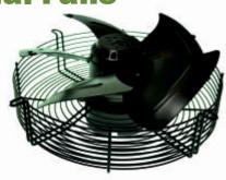
External rotor motor, PSC capacitor. Sucking & blowing airflow. 1PH & 3PH. 2 pole (2700RPM), 4 pole (1350RPM), 6 pole (920RPM) & 8 pole (680RPM). 175mm to 900mm.
