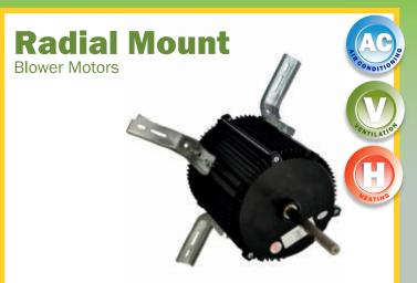
Body diameters include 105, 120, 145mm, etc. 6W to 1100W. Steel shell or extruded aluminium. Single or three speeds. 3 or 4 mounting pads or slots. Uses a blower mounting kit.
