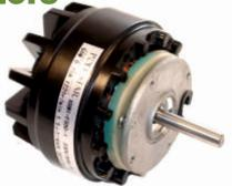
Fitted to 100mm dia. cross flow blowers in fan convectors. 4 pole, 30W & 50W models, ventilated body, single speed,  $4 \times 100$  tapped mounting holes at shaft end, mechanical duty.
