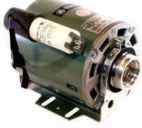
PSC capacitor motor. 180W, 4 pole (1250RPM), ventilated body, intermittent or continuous mechanical duty. Pump drive coupling with cross cut shaft.
