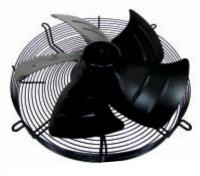
ECM high efficiency motor. Sucking airflow. Diameters: 200, 250, 300, 315, 350, 400 & 450mm. Class B. IP54. 450mm long cable. 1310RPM to 3050RPM. -25'c to +60'c.
