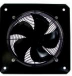
External rotor motor, PSC capacitor. Sucking & blowing airflow. 1PH & 3PH. 2 pole (2700RPM), 4 pole (1350RPM) 6 pole (920RPM) & 8 pole (680RPM). 250mm to 900mm.
